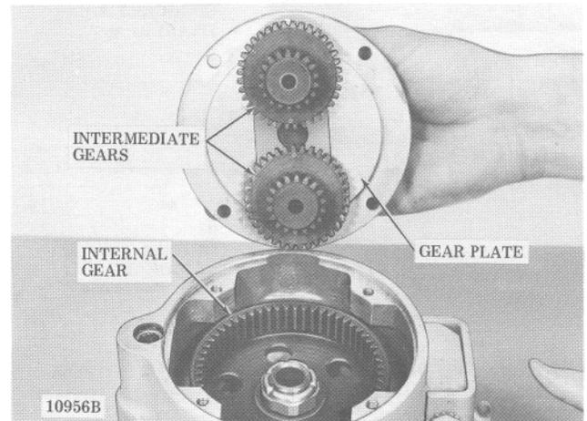
Figure 7-10. Removing Gear Plate and Intermediate Gears.
