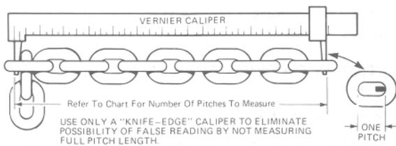
Figure 5-2. Checking Coil Chain Using Vernier Caliper.
