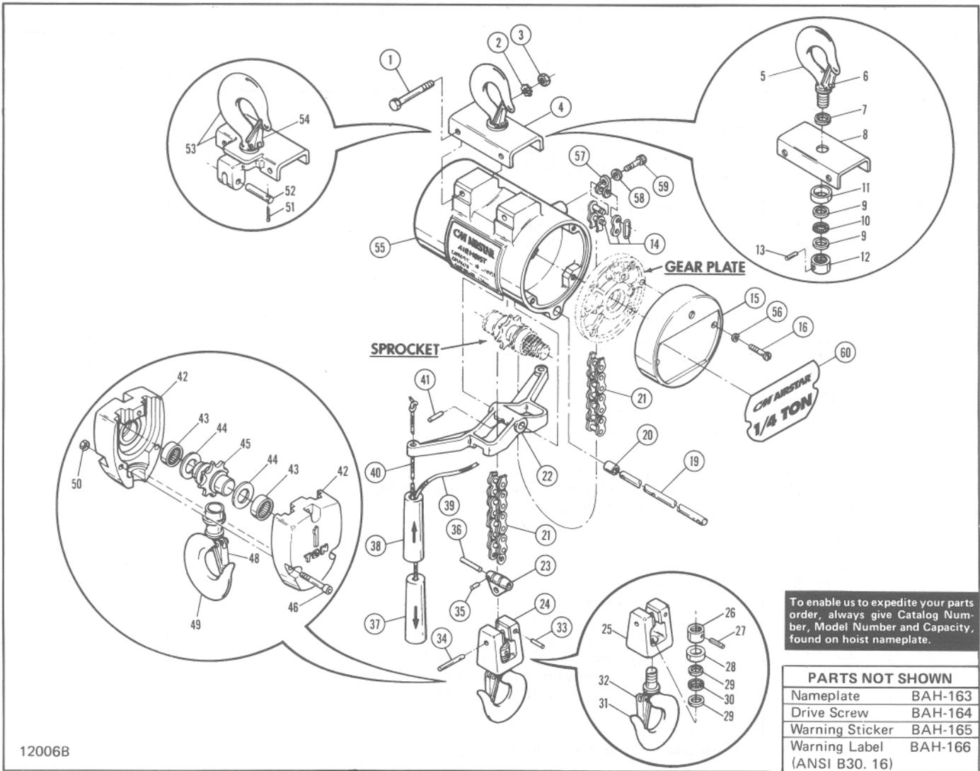
Figure 8-2. Frame and External Parts - Roller Chain Models.
