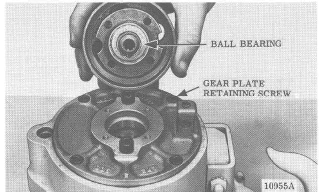
Figure 7-10. Removing Brake Wheel and Ball Bearing Assembly.
